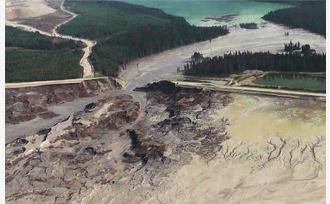
The Imperial Metals Mount Polley gold and copper mine tailings dam disaster in British Columbia, Canada, dumped 24 million cubic meters (more than 31 million cubic yards) in 2014 of mine waste and sludge into neighboring Lake Polley and polluting the Hazelton Creek watershed.
